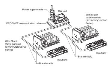
The EX500 range of units can be connected to open fieldbus (PROFINET) to realize the reduction of input or output device wiring and the distributed control syst One branch of manifold valves/input unit can be connected to 32 outputs/32 inputs. Up to 4 branches can be connected (total 128 outputs/128 inputs).
