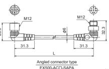
Minimum acceptable cable bending radius: 40 mm (fixed)
