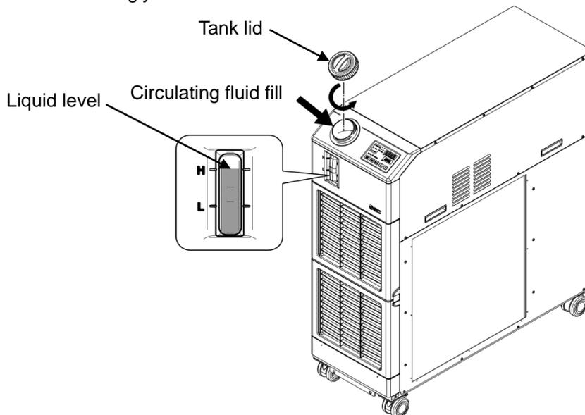
Fig. 3-21 Circulating fluid fill
