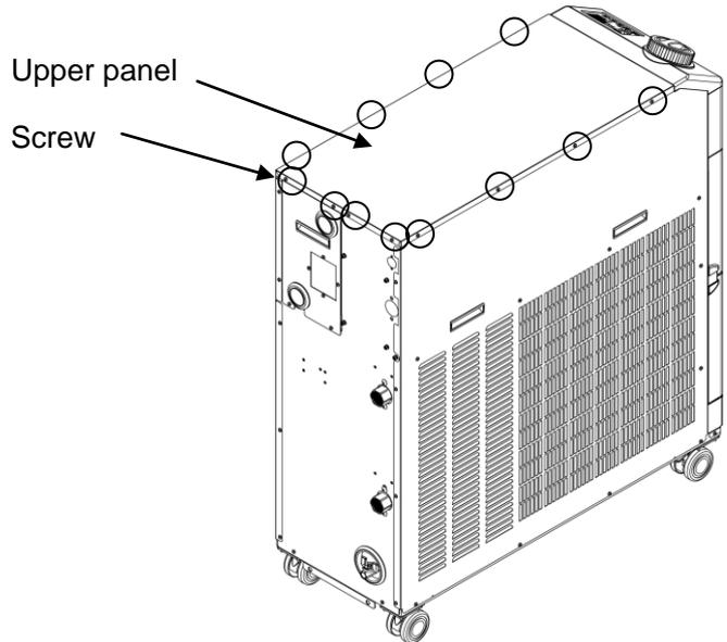
Fig. 7-4 Removal of upper panel
