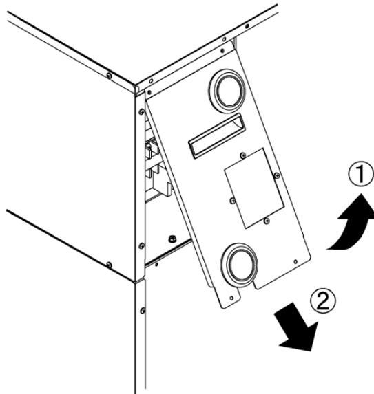
Fig. 3-9 Removal of power supply terminal cover
