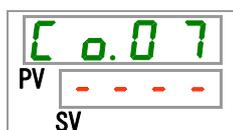
**14.S** Set slave addresses (simple communication protocol) with [▲] key or [▼] key, and press [SEL] key to enter.
