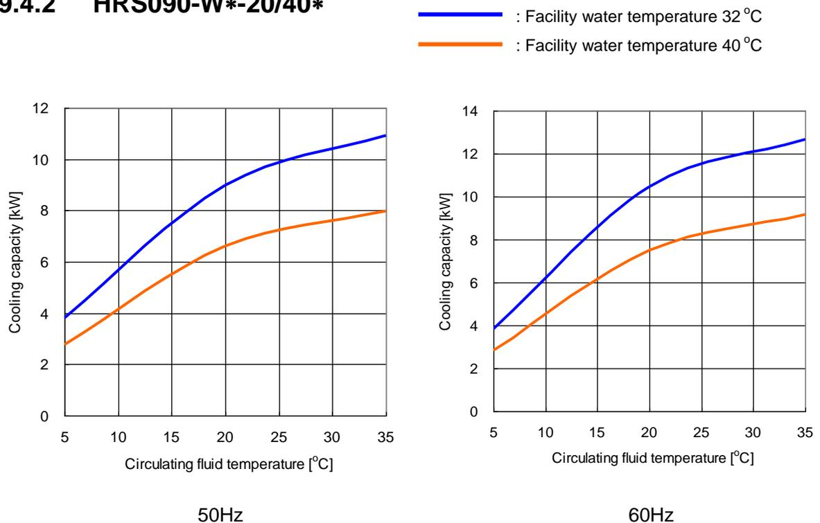
Fig. 9-6 Cooling capacity(HRS090-W\*-20/40\*)
