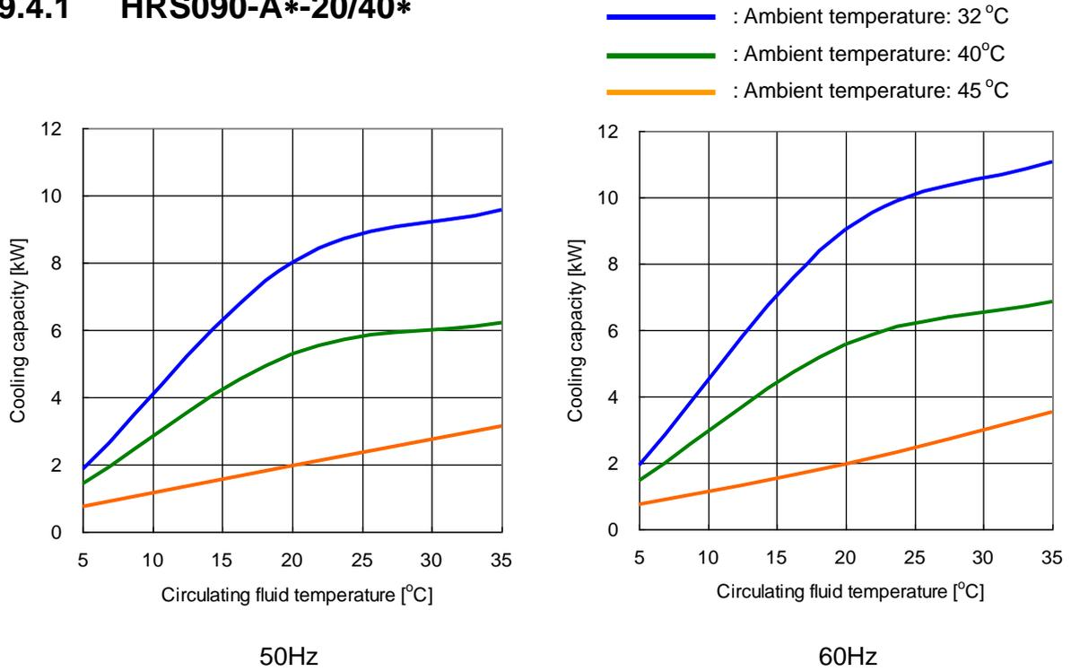
Fig. 9-5 Cooling capacity(HRS090-A\*-20/40\*)
