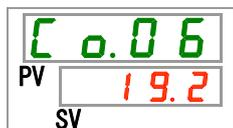
**12.** Set communication speed (MODBUS) with [▲] key or [▼] key, and press [SEL] key to enter.
