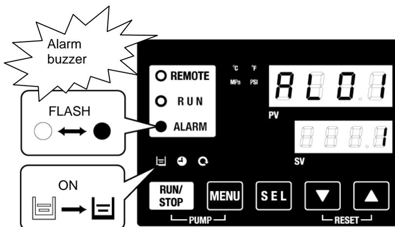
\* [ALARM] light turns ON only when “AL01 Low level in tank” alarm is being generated.
