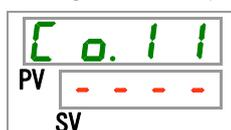
**22.** Perform setting for parity check (simple communication protocol) with [▲] key or [▼] key, and press [SEL] key to enter.
