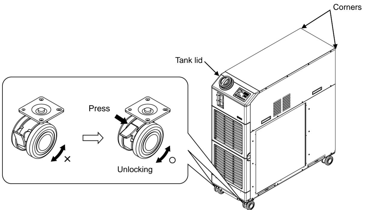
Fig. 3-2 Transportation using casters (This drawing is [HRS090-A-20].)
