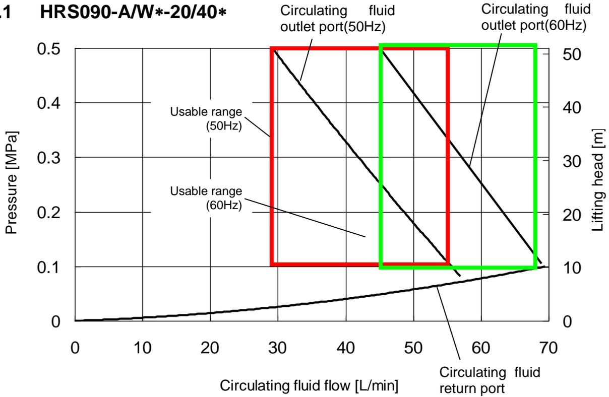
Fig. 9-7 Pump capacity (HRS090-A/W\*-20/40\*)
