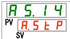
**27.** Set the product operation when "Contact input 2 signal detection" alarm is generated with [▲] key or [▼] key, and press [SEL] key to enter.
