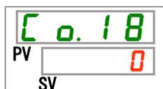
**36.** Set threshold time for the contact input signal 1 OFF detection timer with [▲] key or [▼] key, and press [SEL] key to enter.
