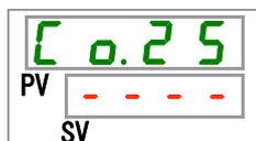
**50.** Set the alarm selected for the contact output signal 1 with [▲] key or [▼] key, and press [SEL] key to enter.
