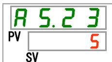
**35.** Set range over detection timer with the [▲] key or [▼] key, and press [SEL] key to enter.
