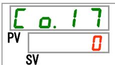
**34.** Set time delay for the contact input signal 1 delay timer for reading with [▲] key or [▼] key, and press [SEL] key to enter.
