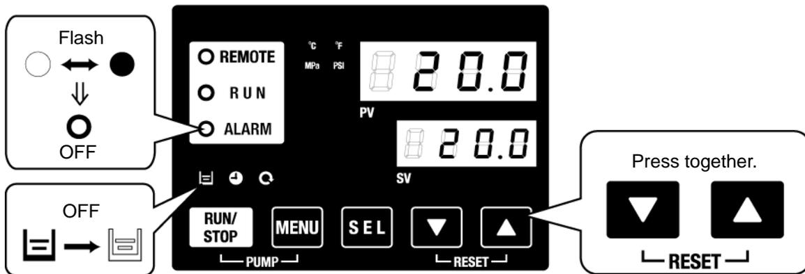
\* [ALARM] light turns ON only when "AL01 Low level in tank" alarm is being generated.
