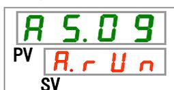
**17.** Set the product operation when "Circulating fluid discharge pressure drop" alarm is generated with [▲] key or [▼] key, and press [SEL] key to enter.
