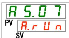
**13.** Set the product operation when "Circulating fluid discharge pressure rise" alarm is generated with [▲] key or [▼] key, and press [SEL] key to enter.
