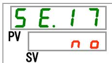
**9.** Select **YES** with [▲] key or [▼] key, and press [SEL] key to enter. Select **YES** and press [SEL] key to enter, and the accumulated operating time of the compressor will be reset. The display returns to the main menu.
