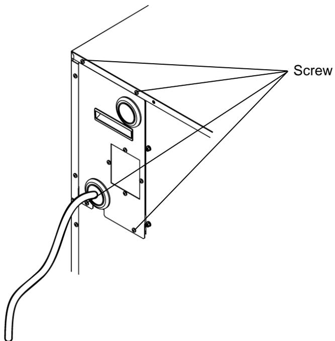
Fig. 3-12 Mounting of power supply terminal cover
