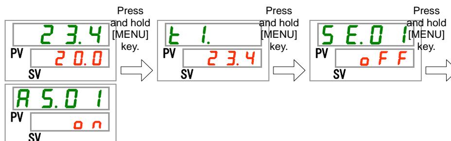
Setting/Checking: Alarm buzzer sound
