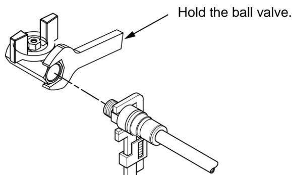
Fig. 3-19 Connection to the drain
