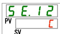
3. Select a temperature unit with [▲] key or [▼] key, and press [SEL] key to enter.
