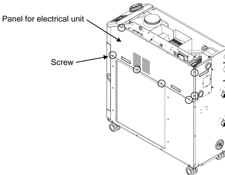
Fig. 7-2 Remove the panel of the electrical unit
