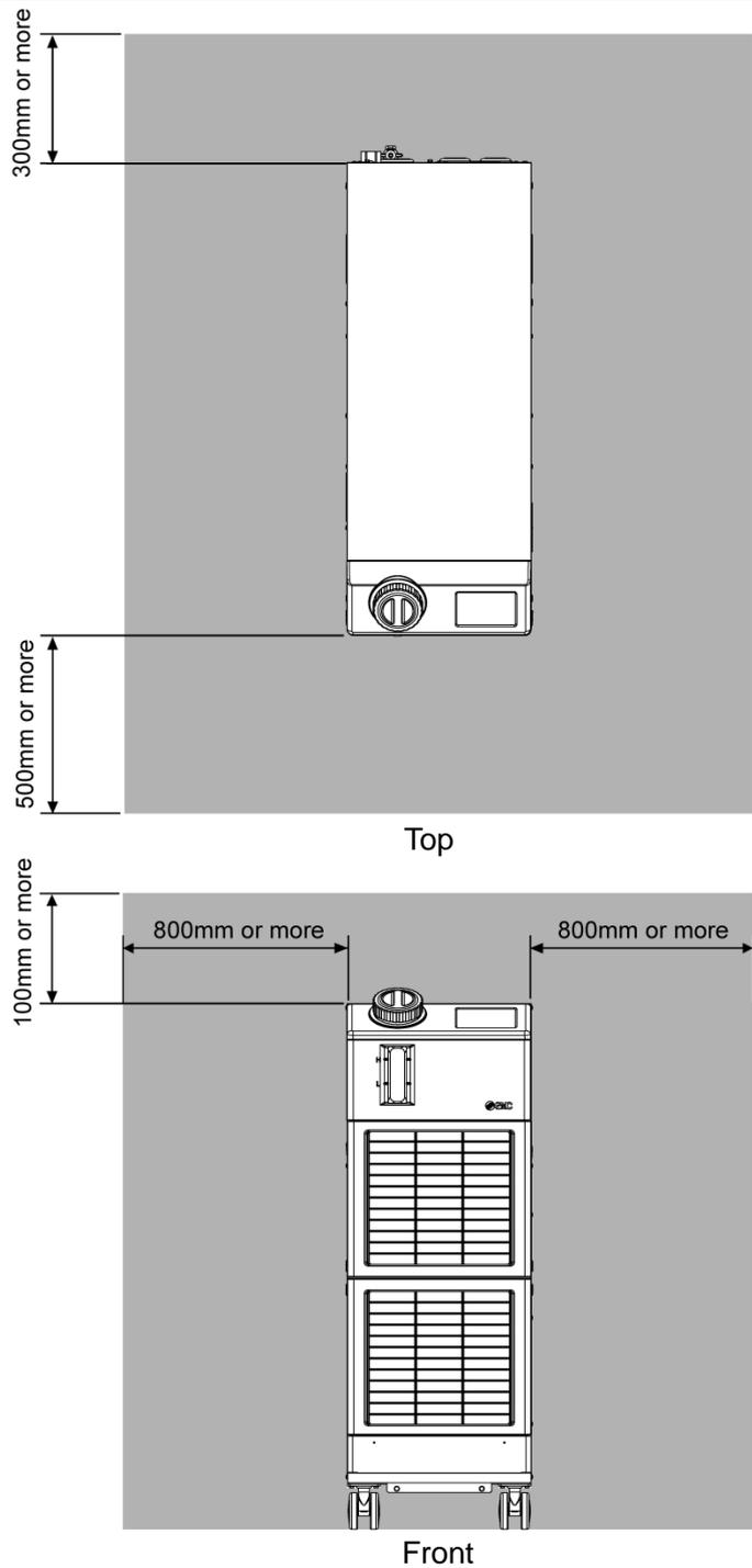
Fig. 3-3 Installation space (This drawing is [HRS090-A-20].)
