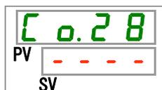
**56.** Set the alarm selected for the contact output signal 2 with [▲] key or [▼] key, and press [SEL] key to enter.
