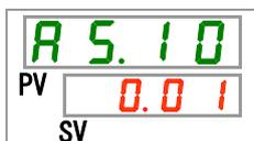
**19.** Set the threshold detection pressure for "Circulating fluid discharge pressure drop" alarm generation with [▲] key or [▼] key, and press [SEL] key to enter.
