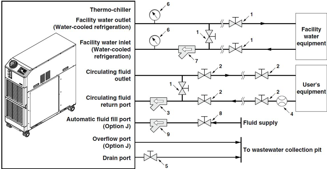
Fig. 3-20 Recommended piping circuit
