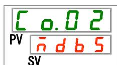
4. Select a serial communication protocol with [▲] key or [▼] key, and press [SEL] key to enter.
