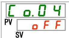
8. Perform a setting of terminal for RS-485 with [▲] key or [▼] key, and press [SEL] key to enter.
