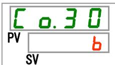
**60.** Set the operation type of the contact output signal 3 with [▲] key or [▼] key, and press [SEL] key to enter.
