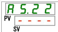
**33.** Set monitoring start timer with the [▲] key or the [▼] key, and press [SEL] key to enter.
