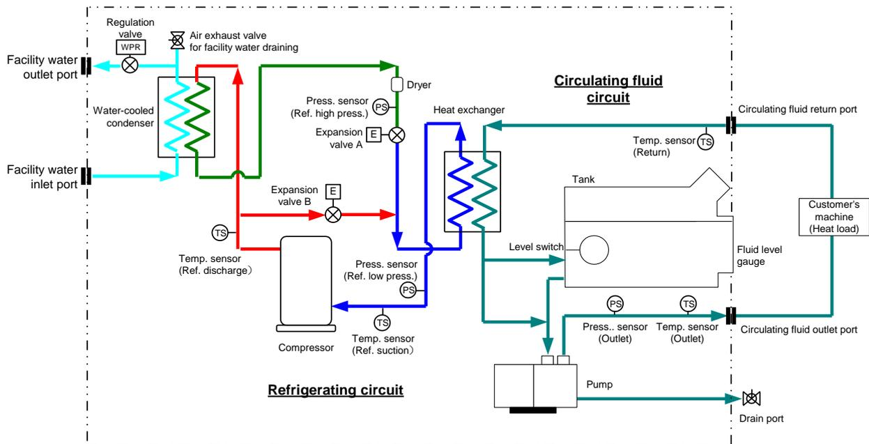
Fig. 9-4 Flow diagram(HRS090-W\*-20/40\*)
