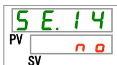
3. Select  YES with [▲] button or [▼] button, and press [SEL] button to enter. Select  YES and press [SEL] button to enter. This resets all the data to the default, and the display returns to the main display.
