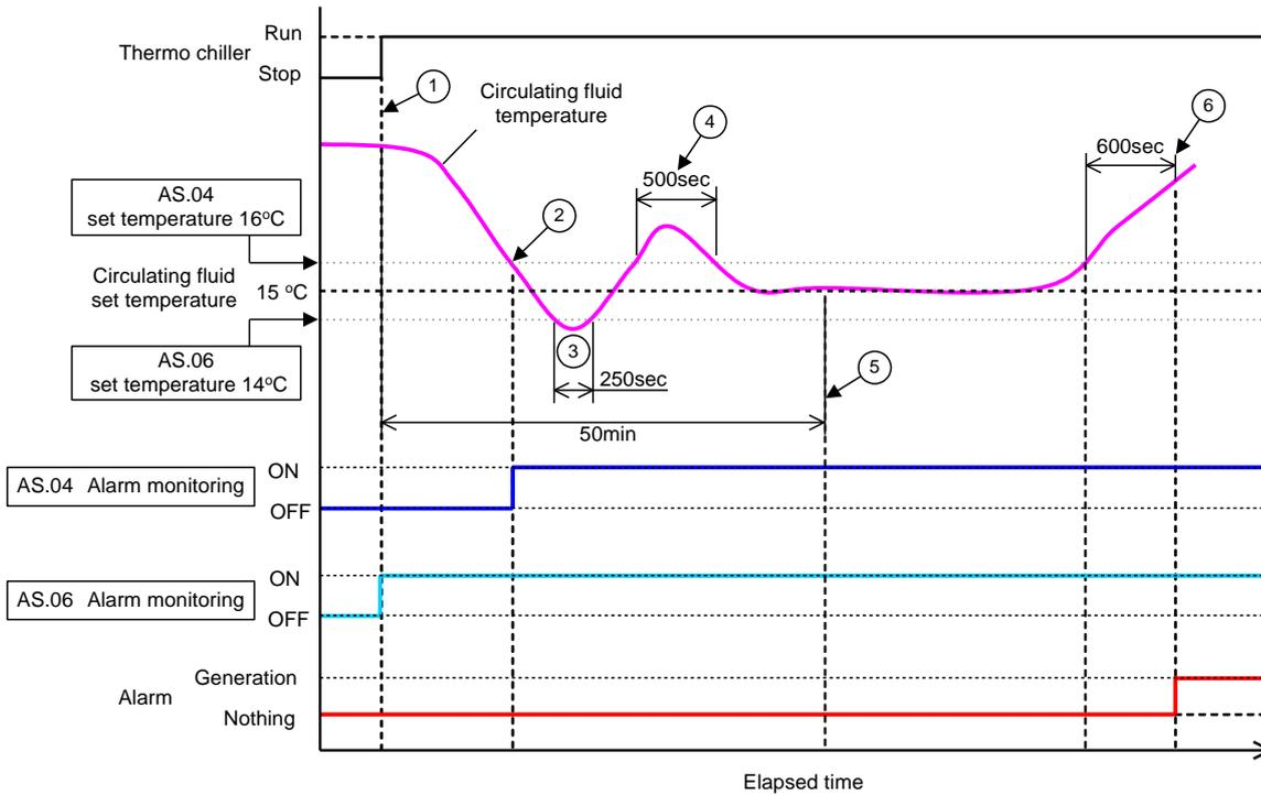
Fig 5-4 Alarm generation timing
