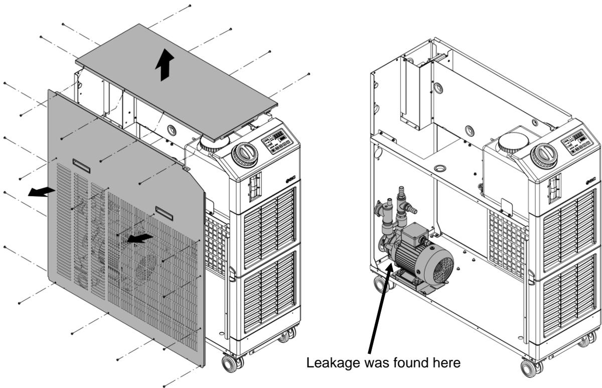
Fig. 8-3 Check for water leakage from pump
