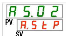
3. Set the product operation when "Low level in tank" alarm is generated with [▲] key or [▼] key, and press [SEL] key to enter.
