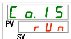
**30.** Perform setting for the contact input signal 1 with [▲] key or [▼] key, and press [SEL] key to enter.
