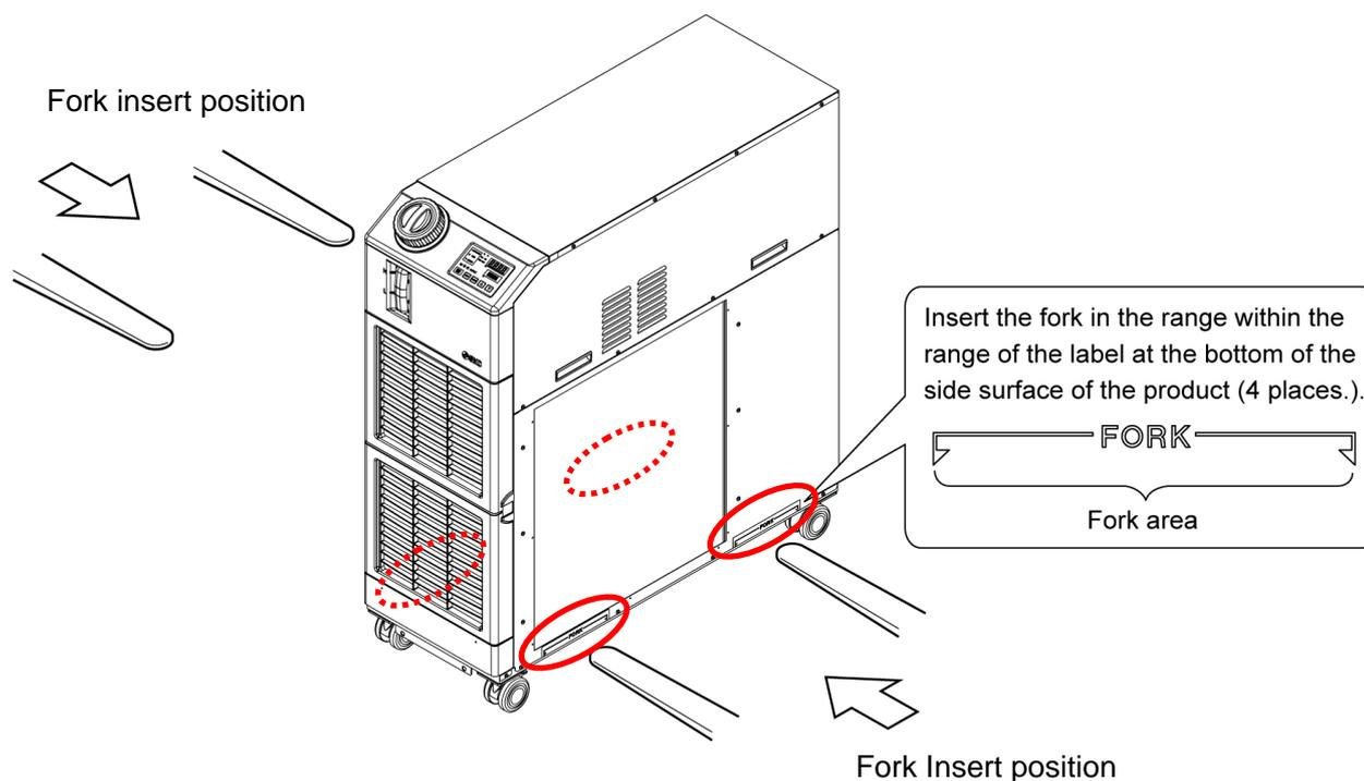
Fig 3-1 Fork inserting and hanging position (This drawing is [HRS090-A-20].)
