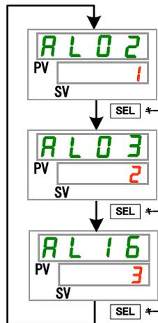
The alarm code displayed on the operation panel is AL02. AL03 and AL16 are displayed by pressing the [SEL] button.
