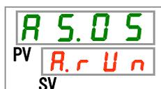
**9.** Set the product operation when "Circulating fluid discharge temp. drop" alarm is generated with [▲] key or [▼] key, and press [SEL] key to enter.
