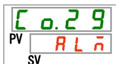
**58.** Select a function for the contact output signal 3 with [▲] key or [▼] key, and press [SEL] key to enter.
