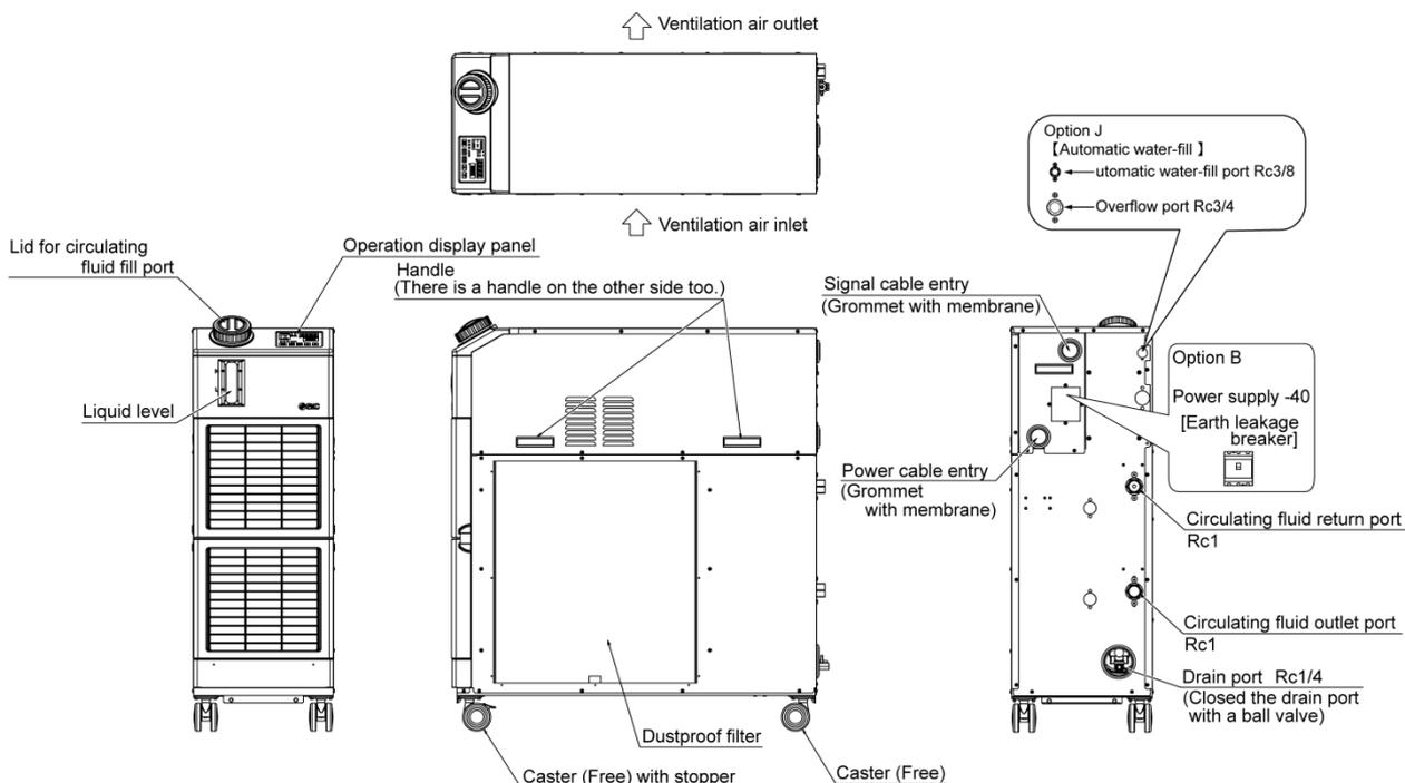
Fig. 2-2 Names of the parts (This drawing shows “HRS090-A-20”.)
