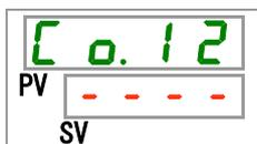
**24.** Set stop bit (simple communication protocol) with [▲] key or [▼] key, and press [SEL] key to enter.
