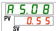
**15.** Set the threshold detection pressure for "Circulating fluid discharge pressure rise" alarm generation with [▲] key or [▼] key, and press [SEL] key to enter.
