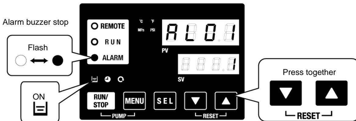
\* [AL] light turns ON only when “AL01 Low level in tank” alarm is being generated.
