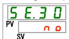
**12.** Select **YES** with [▲] key or [▼] key, and press [SEL] key to enter. Select **YES** and press [SEL] key to enter, and the accumulated operating time of the dust-proof filter will be reset. The display returns to the main menu.
