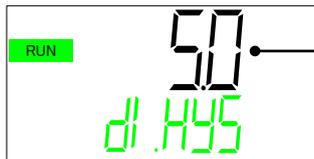
Electric conductivity control hysteresis set value Unit:  $\mu\text{S} / \text{cm}$
