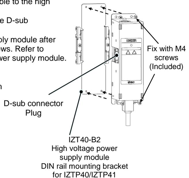
III. When the high voltage power supply module is added directly
