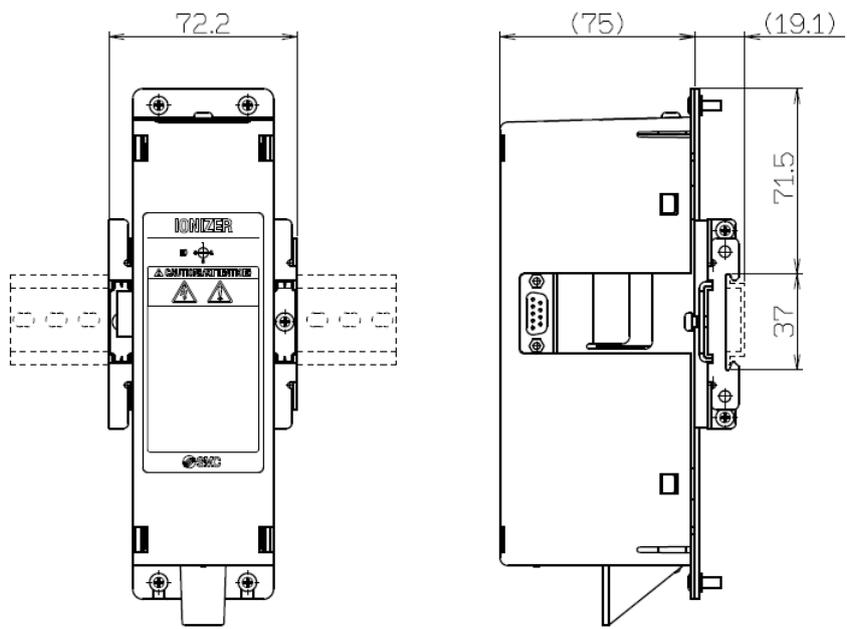
High voltage power supply module (IZTP42)
