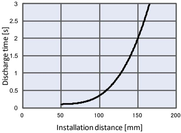
2) With High speed static neutralization cartridge
