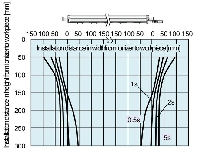
4) With Energy saving high-efficiency cartridge, Supply pressure: 0.3 MPa
