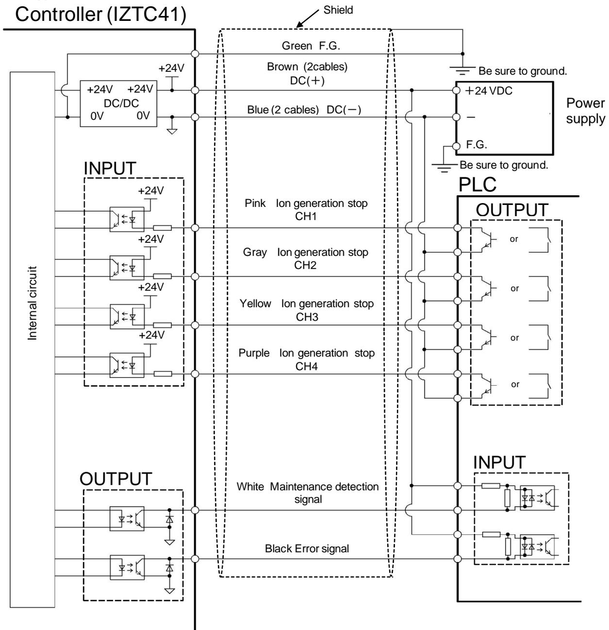
When an ionizer (IZT41) is used in DC mode, make sure to ground the F.G. cable (green) and DC(-) cable (blue) of the input power supply **with a resistance of 100 ohms or less**. Without grounding the DC(-) cable, this products and/or power supply may be damaged.
