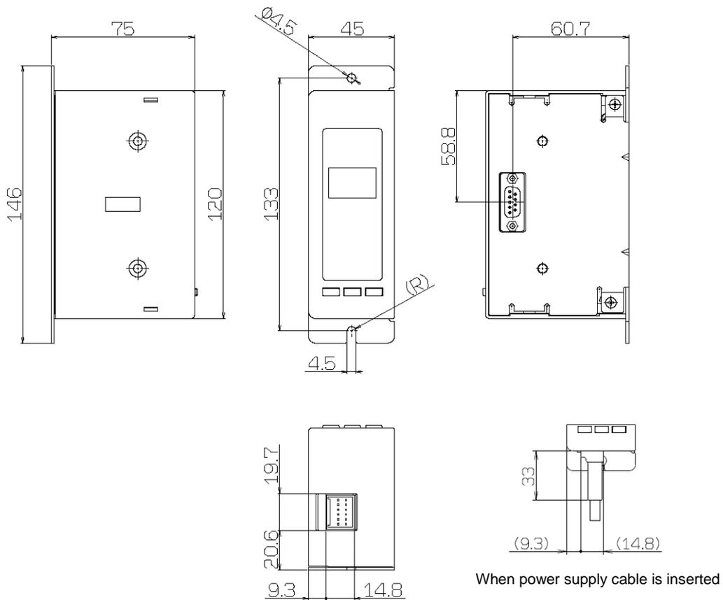
When DIN rail mounting bracket (IZT40-B1) is used
