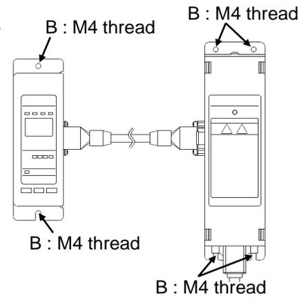
III. Adding a high voltage power supply module
