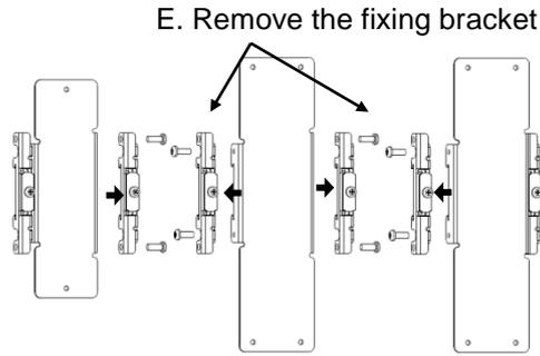
b. Mounting of DIN rail mounting bracket
