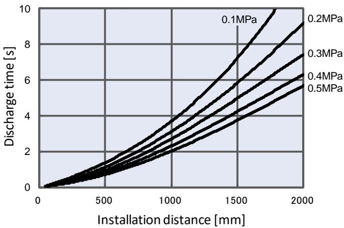
4) With Energy saving high-efficiency cartridge
