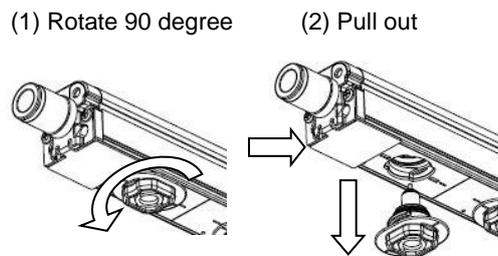
Removal procedure of emitter cartridge
