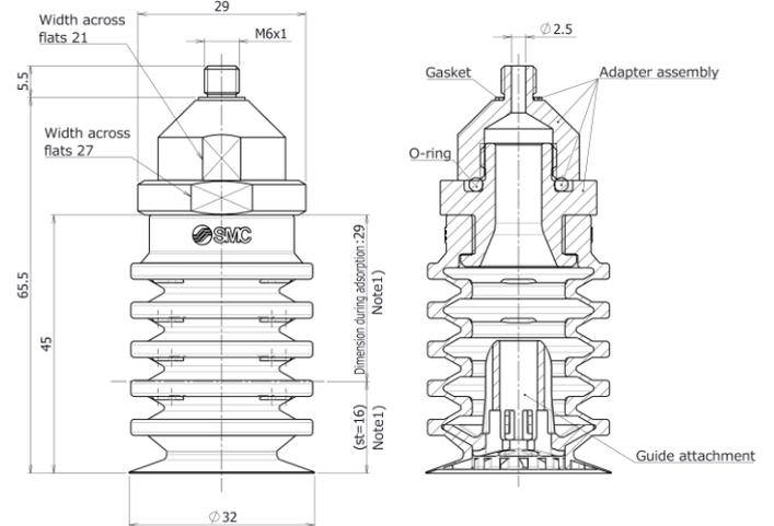
Note1) "D" and (st) indicate the reference value during adsorption at vacuum pressure: -85[kPa].
