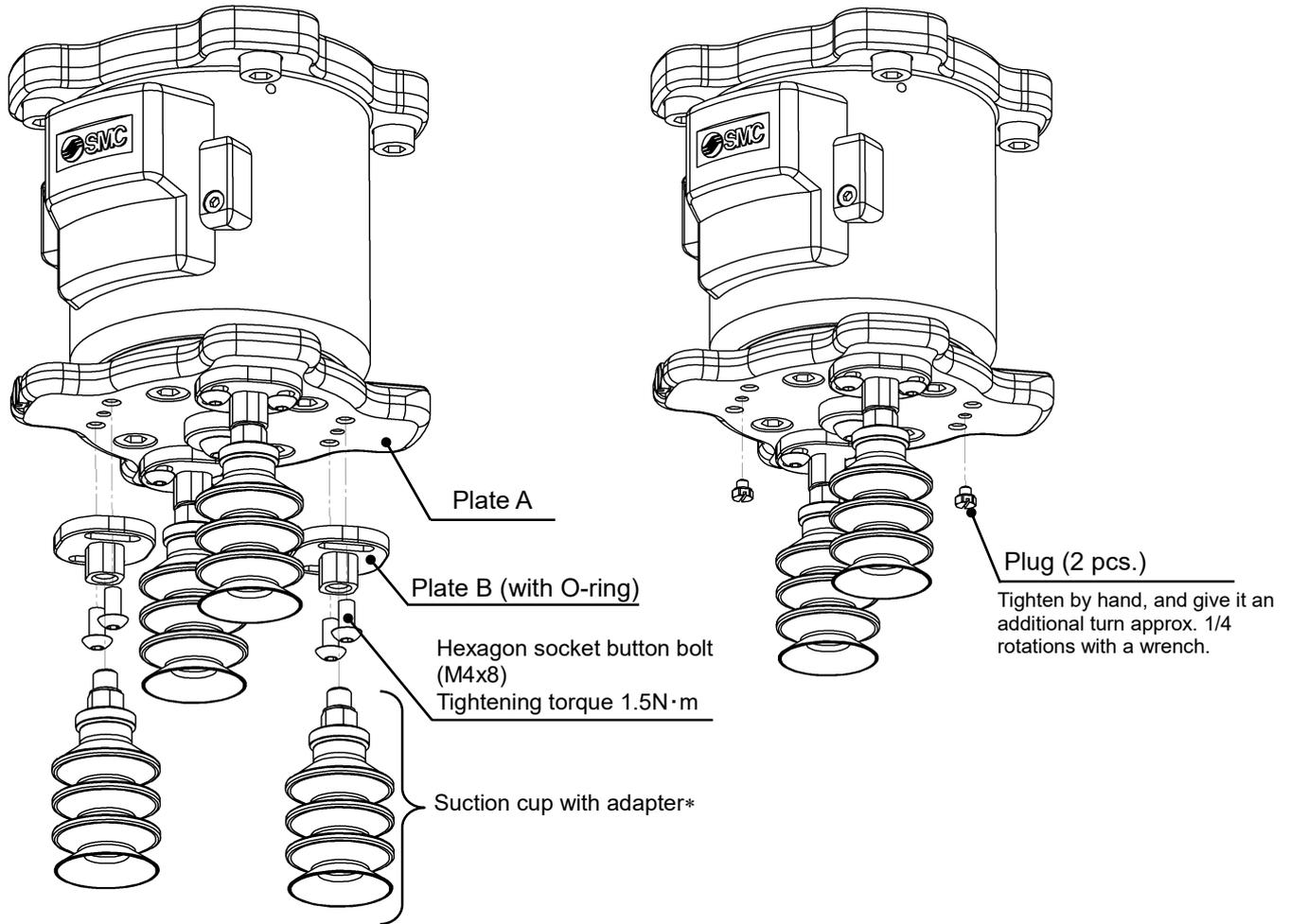
(1) Disassemble the suction cups with adapter
