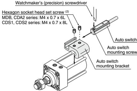
1. Fix it to the detecting position with a set screw by installing an auto switch mounting bracket in cylinder tie-rod and letting the bottom surface of an auto switch mounting bracket contact the cylinder tube firmly.
