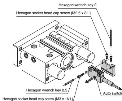
1. Insert the hexagon socket head cap screw (M2.5 x 0.45 x 8 L) down lightly to the M2.5 tapped portion of the lower part of auto switch mounting bracket's concave part. (2 locations) Use caution to avoid the tip of a screw from sticking out of the auto switch mounting bracket's bottom surface.
