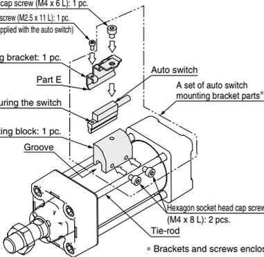
\* Brackets and screws enclosed by a dashed line are a set of auto switch mounting bracket parts.
