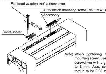
Note) When tightening an auto switch mounting screw, use a watchmaker's screwdriver with a grip diameter of 5 to 6 mm. Also, set the tightening torque to be 0.05 to 0.1 N·m. As a guide, turn 90° from the position where it comes to feel tight.
