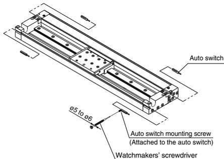
(Note) When tightening an auto switch mounting screw, use a watchmaker's screwdriver with a grip diameter of 5 to 6 mm. The tightening torque should be about 0.05 to 0.1 N·m.
