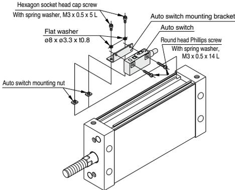
1. From the cutoff part of the rail on the cylinder body, insert the auto switch mounting nuts (2 pcs.) into the rail groove.
