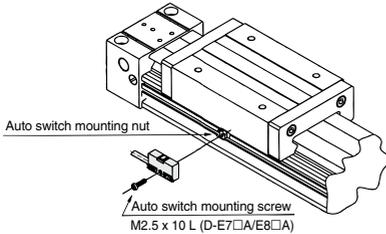
1. Insert the auto switch mounting nut into the auto switch mounting groove and then set the auto switch at the mounting position by sliding.
