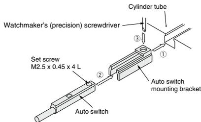
1. Insert the auto switch mounting bracket into the auto switch mounting groove to set it roughly to the auto switch mounting position.
