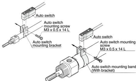
1. For **CDJ2 series**: Put a mounting bracket on the cylinder tube.
