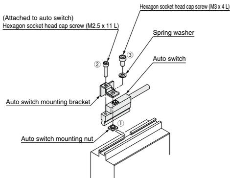
1. Insert the auto switch mounting nut into the groove on the auto switch mounting rail.
