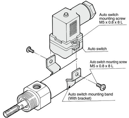
1. Tighten completely the auto switch mounting screw on the auto switch body side.
