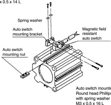
1. Mount the auto switch mounting bracket onto the auto switch mounting nut by tightening bracket fixing screw lightly through the mounting hole on the top of bracket.
