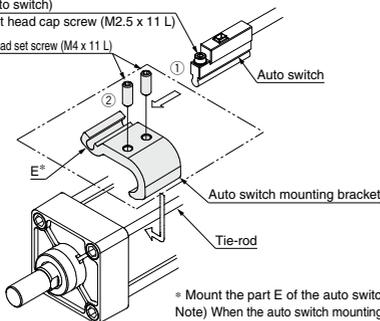
\* Mount the part E of the auto switch mounting bracket so that it is in contact with the cylinder tube.
