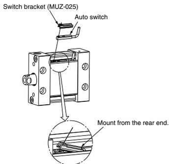
\* It is recommended to mount the switch bracket from the rear end.
