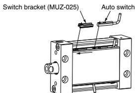
1. First, push the switch bracket into the switch groove.
