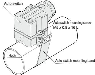
1. Loosen the auto switch mounting screws at both sides to pull down the hook.
