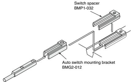
1. After picking up a switch spacer between your fingers, push it into the cylinder tube groove.
