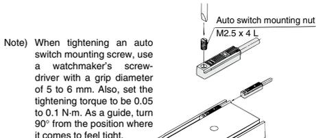
Note) When tightening an auto switch mounting screw, use a watchmaker's screwdriver with a grip diameter of 5 to 6 mm. Also, set the tightening torque to be 0.05 to 0.1 N·m. As a guide, turn 90° from the position where it comes to feel tight.
