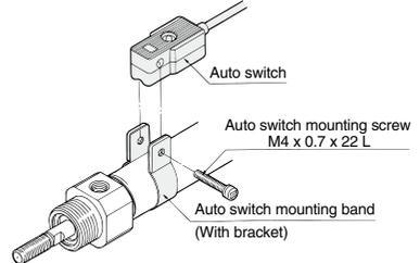
1. Put a mounting band on the cylinder tube and set it at the auto switch mounting position.
