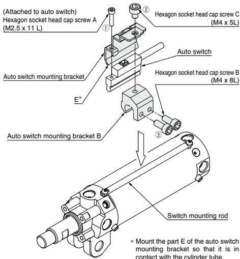
1. Remove the hexagon socket head cap screw A (M2.5) that is attached to the auto switch. Mount the auto switch mounting bracket (pressed stainless steel bracket) on the auto switch and tighten the hexagon socket head cap screw A (M2.5) you have removed 3 to 4 turns to temporarily mount the bracket.
