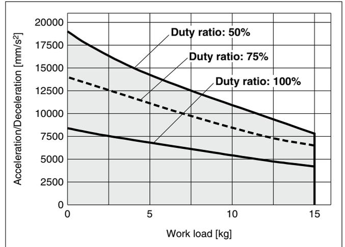
**Work Load–Acceleration/Deceleration Graph (Guide)**
