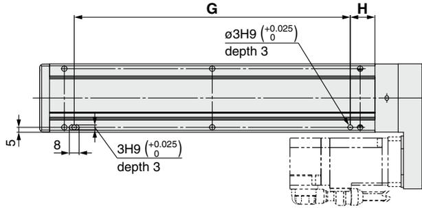
\*1 When using the body bottom positioning pin holes, do not simultaneously use the housing B bottom pin hole.
