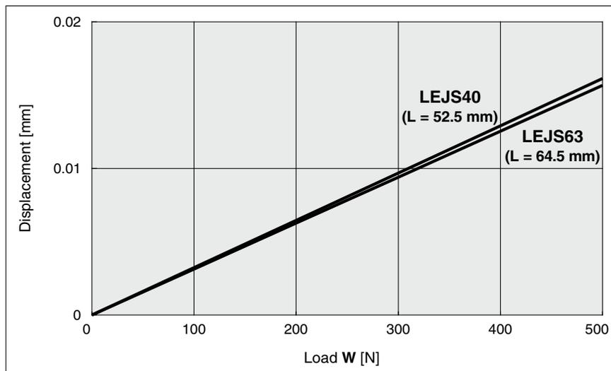
\* This displacement is measured when a 15 mm aluminum plate is mounted and fixed on the table. (Table clearance is included.)
