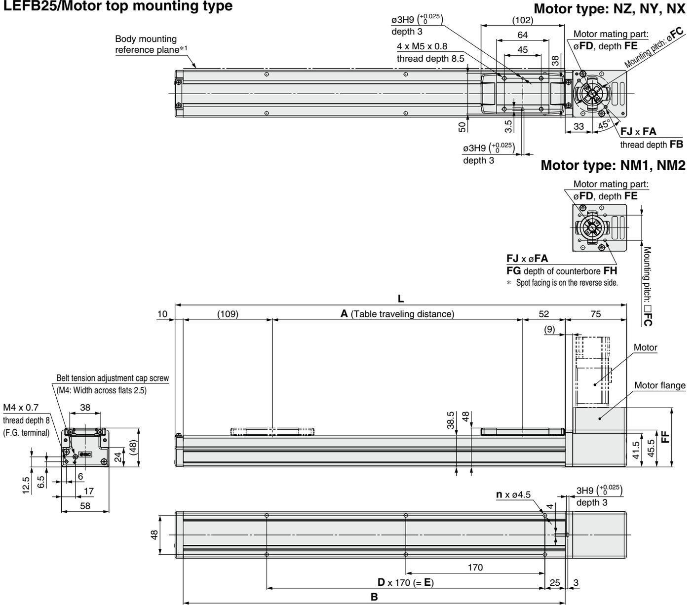
\*1 When mounting the actuator using the body mounting reference plane, set the height of the opposite surface or pin to be 3 mm or more. (Recommended height 5 mm)
