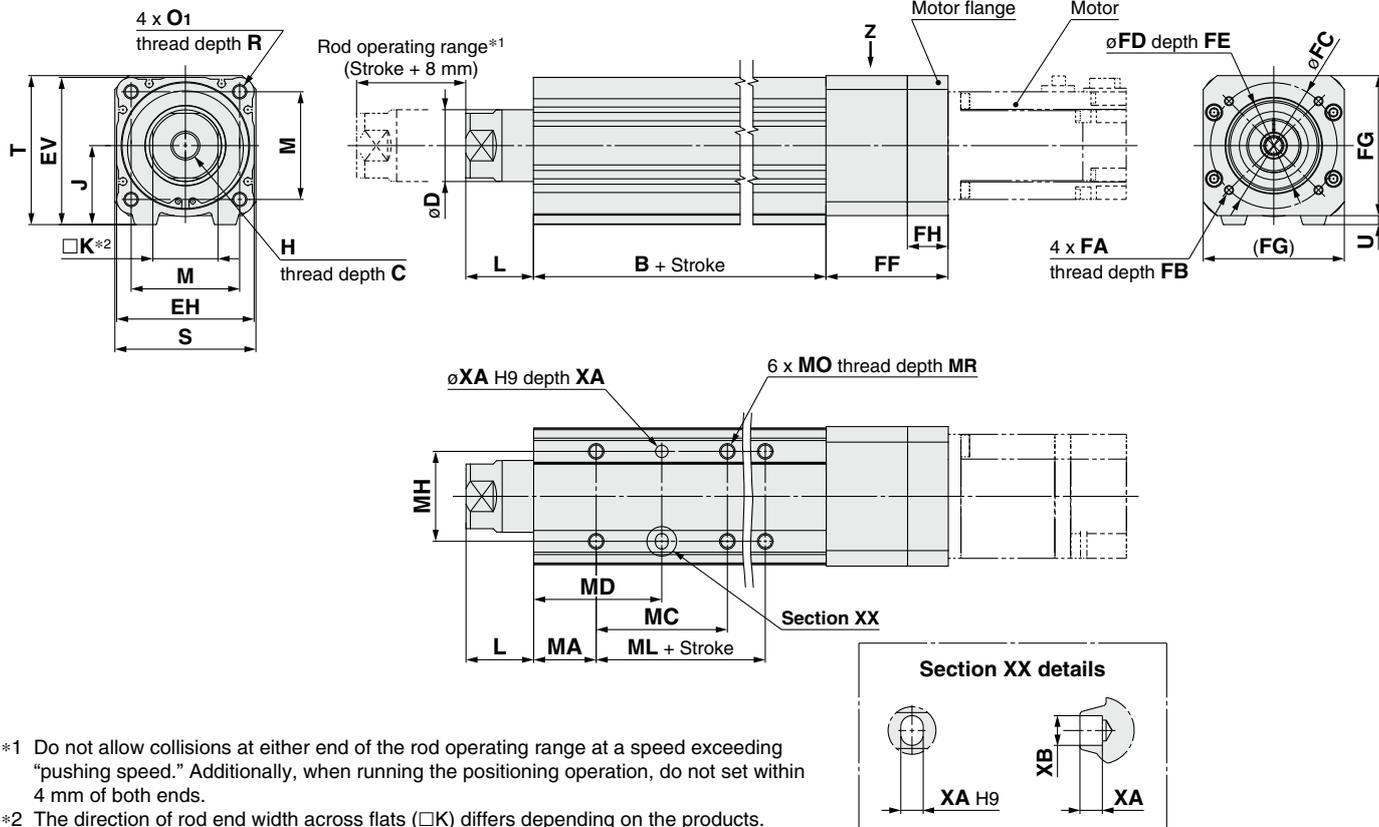
\*1 Do not allow collisions at either end of the rod operating range at a speed exceeding "pushing speed." Additionally, when running the positioning operation, do not set within 4 mm of both ends.
