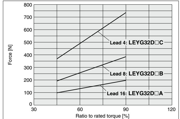
\* When using the force control or speed control, set the maximum value to be no more than 90% of the rated torque.
