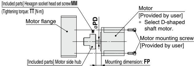
\* Note for mounting a hub to the NM1 motor type
