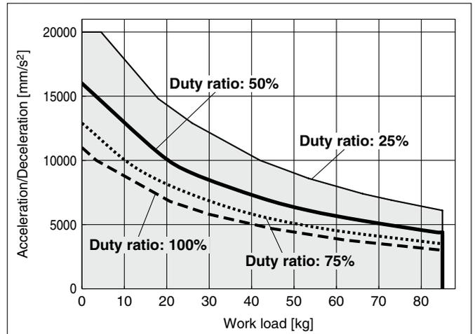
These graphs are examples of when the standard motor is mounted.
