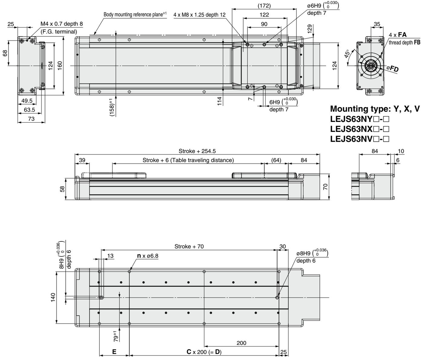
\*1 When mounting the actuator using the body mounting reference plane, use a pin. Set the height of the pin to be 5 mm or more because of round chamfering. (Recommended height 6 mm)
