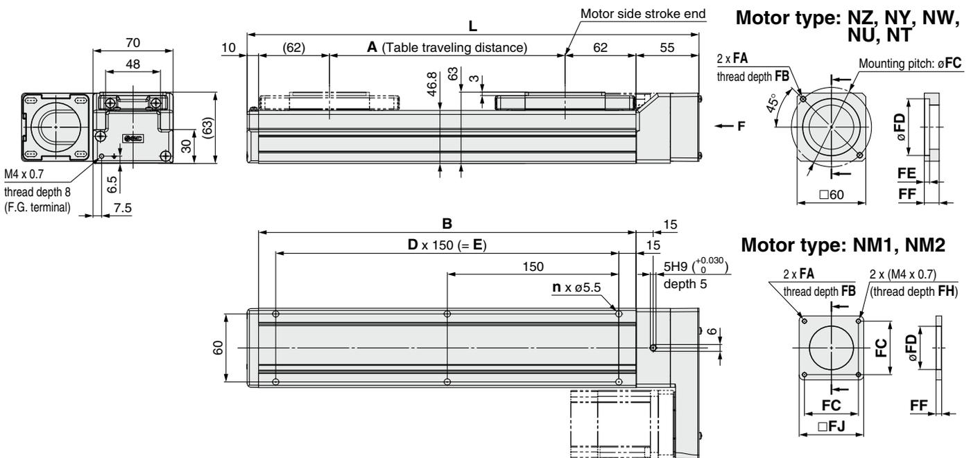
\*1 When mounting the actuator using the body mounting reference plane, set the height of the opposite surface or pin to be 3 mm or more. (Recommended height 5 mm)
