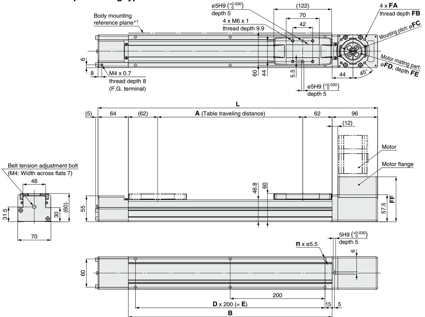
\*1 When mounting the actuator using the body mounting reference plane, set the height of the opposite surface or pin to be 3 mm or more. (Recommended height 5 mm)
