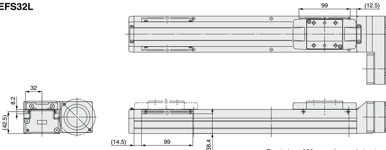
\* For strokes of 99 mm or less, only 1 auto switch mounting bracket can be installed on the motor side.
