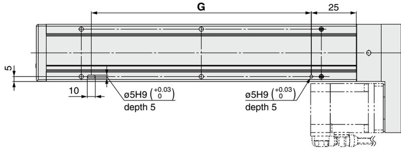
\*1 When using the body bottom positioning pin holes, do not simultaneously use the housing B bottom pin hole.
