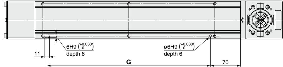
\*1 When using the body bottom positioning pin holes, do not simultaneously use the housing B bottom pin hole.
