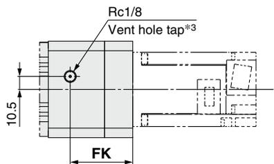
\*3 When using the dust-tight/water-jet-proof (IP65 equivalent), correctly mount the fitting and tubing to the vent hole tap, and then place the end of the tubing in an area not exposed to dust or water. The fitting and tubing should be provided separately by user. Select [Applicable tubing O.D.: ø4 or more, Connection thread: Rc1/8].
