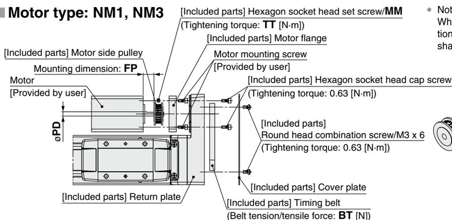
\* Note for mounting a pulley to the NM1 and NM3 motor type
