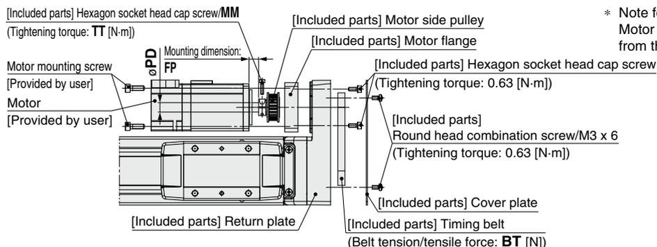
\* Note for mounting a motor to the NM2 motor type
