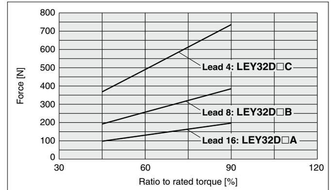
\* When using the force control or speed control, set the maximum value to be no more than 90% of the rated torque.
