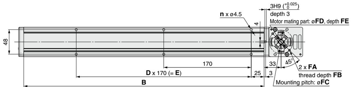
Motor type: NM1, NM2
