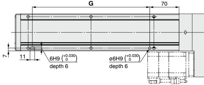
\*1 When using the body bottom positioning pin holes, do not simultaneously use the housing B bottom pin hole.
