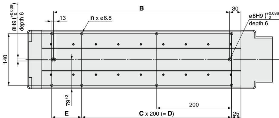
\*3 When mounting the actuator using the body mounting reference plane, use a pin. Set the height of the pin to be 5 mm or more because of round chamfering. (Recommended height 6 mm)
