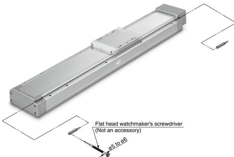
\* When tightening the auto switch mounting screw (included with auto switch), use a watchmaker's screwdriver with a handle diameter of about 5 to 6 mm.
