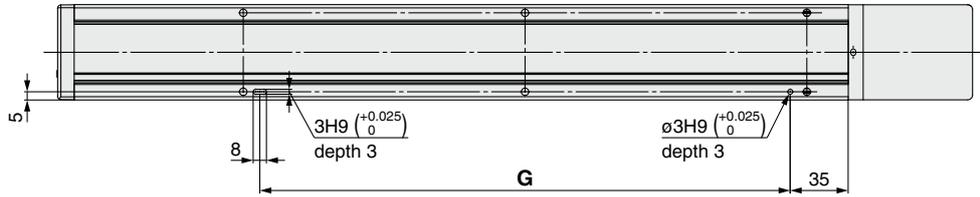
\*1 When using the body bottom positioning pin holes, do not simultaneously use the housing B bottom pin hole.
