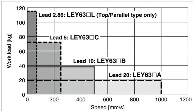
\* The values shown below are allowable values of the actuator body. Do not use the actuator so that it exceeds these specification ranges.
