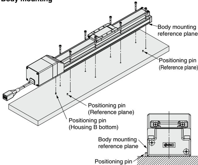
The traveling parallelism is the reference plane for the body mounting reference plane. If the traveling parallelism for a table is required, set the reference plane against parallel pins, etc.
