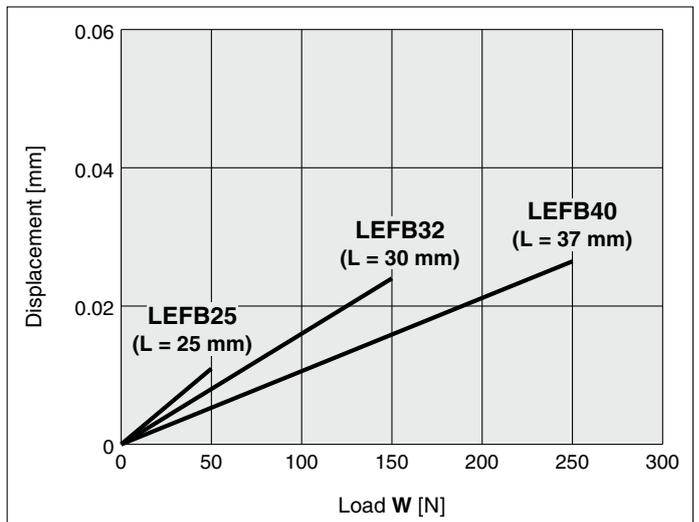
\* This displacement is measured when a 15 mm aluminum plate is mounted and fixed on the table.
