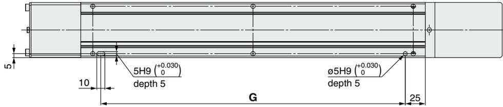
\*1 When using the body bottom positioning pin holes, do not simultaneously use the housing B bottom pin hole.
