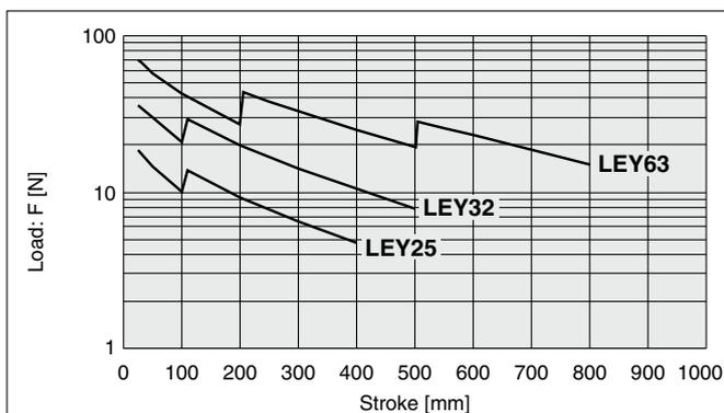
$$[\text{Stroke}] = [\text{Product stroke}] + [\text{Distance from the rod end to the center of gravity of the workpiece}]$$
