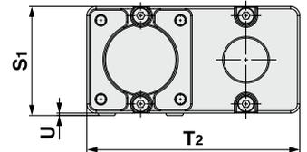
\* When the motor is mounted on the left or right side in parallel, the groove for auto switch on the side to which the motor is mounted is hidden.
