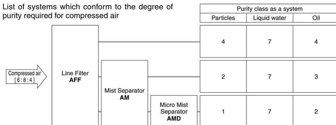
The class indicates the compressed air purity according to ISO 8573-1:2010 (JIS B 8392-1:2012) and indicates the maximum purity class which can be obtained using that system. Note, however, that this value will differ according to the inlet air conditions.
