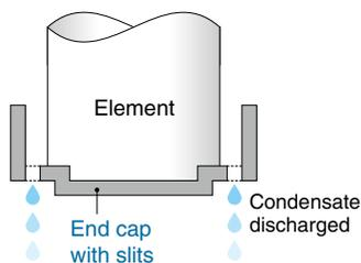
Condensate is not accumulated so no water flows to the downstream side.
