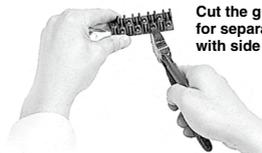
Cut the groove for separation with side cutters.
