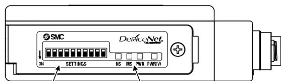
Switch for setting of the address and the baud rate
