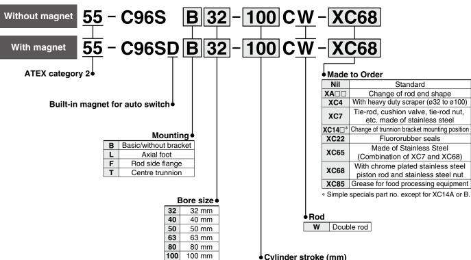
Cylinder stroke (mm)
