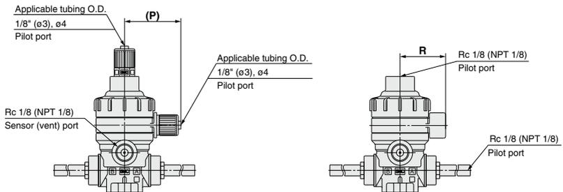
LVQ□<sub>2</sub>-T□ Dimensions (N.O. Valve, Double Acting Valve) (mm)
