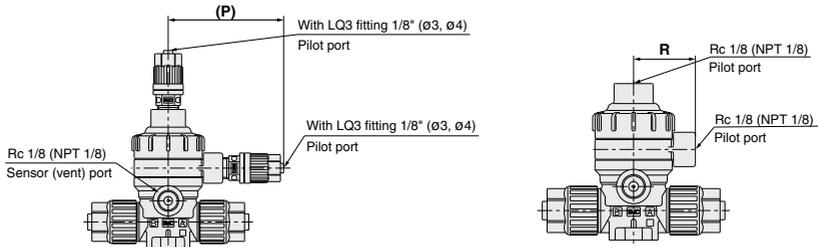
**LVQ□<sub>2</sub>-Z□□□ Dimensions (N.O. Valve, Double Acting Valve)**
