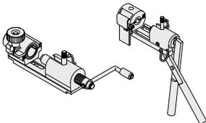
2. Tighten the nut until it touches the end surface of the body, and then tighten it an additional 1/8 turn. If the nut won't turn any further, then it means a sufficient tightening has occurred. Refer to the proper tightening torques shown below.
