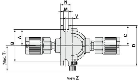
Dimensions (N.O Valve, Double Acting Valve) (mm)
